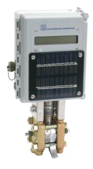
The XALCR™ is an economical replacement for aging circular chart recorders. The XALCR™ comes complete with an integrated multivariable transmitter for Differential Pressure, Static Pressure, and a 6 ft. Temperature Probe. Data can be read locally on the LCD display or collected with Field Manager™. The circular charting feature allows users to display data graphically, similar to a chart recorder.
